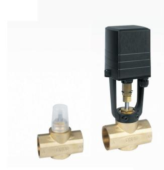
Electric Control Valve assemble with 1200N force actuator and valve size from DN20 to DN65, which widely used in air conditioning, refrigeration, heating and building automation system, can adjust the medium flow precision, achieved goal to control temperature, humidity, pressure and energy saving.
